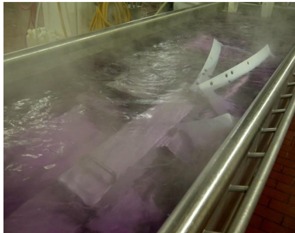
Fig. 19. Equipment must be fully submerged for appropriate cleaning
