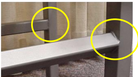
Fig. 11. The square tubing on the left will accumulate soil on the flat horizontal surface. By rotating 90°, or using round tubing, flat surfaces are minimized.
