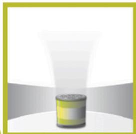
The active substance rises, allowing the operator time to leave the room. It is propelled by slow, non-pyrotechnic combustion.
